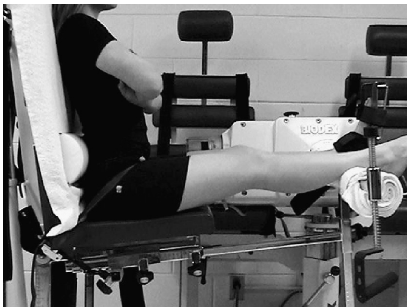
Fig. 5. Upright sitting position illustrating the foam wedge used to impose an anterior pelvic posture.
